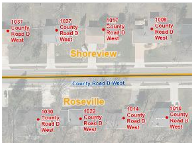
Figure 5-8 Coincident Road Centerline and Jurisdiction Boundaries
